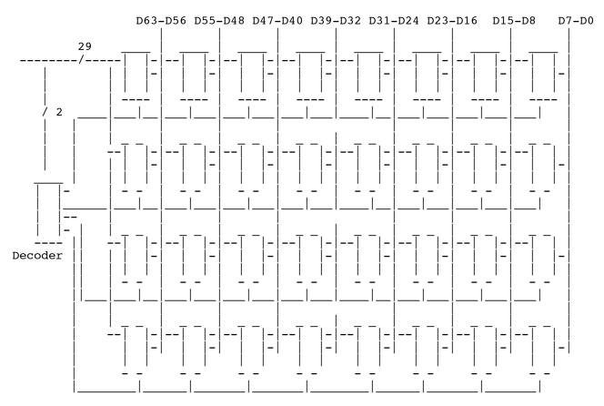
a. Each chip connects to four bit of the data bus.
